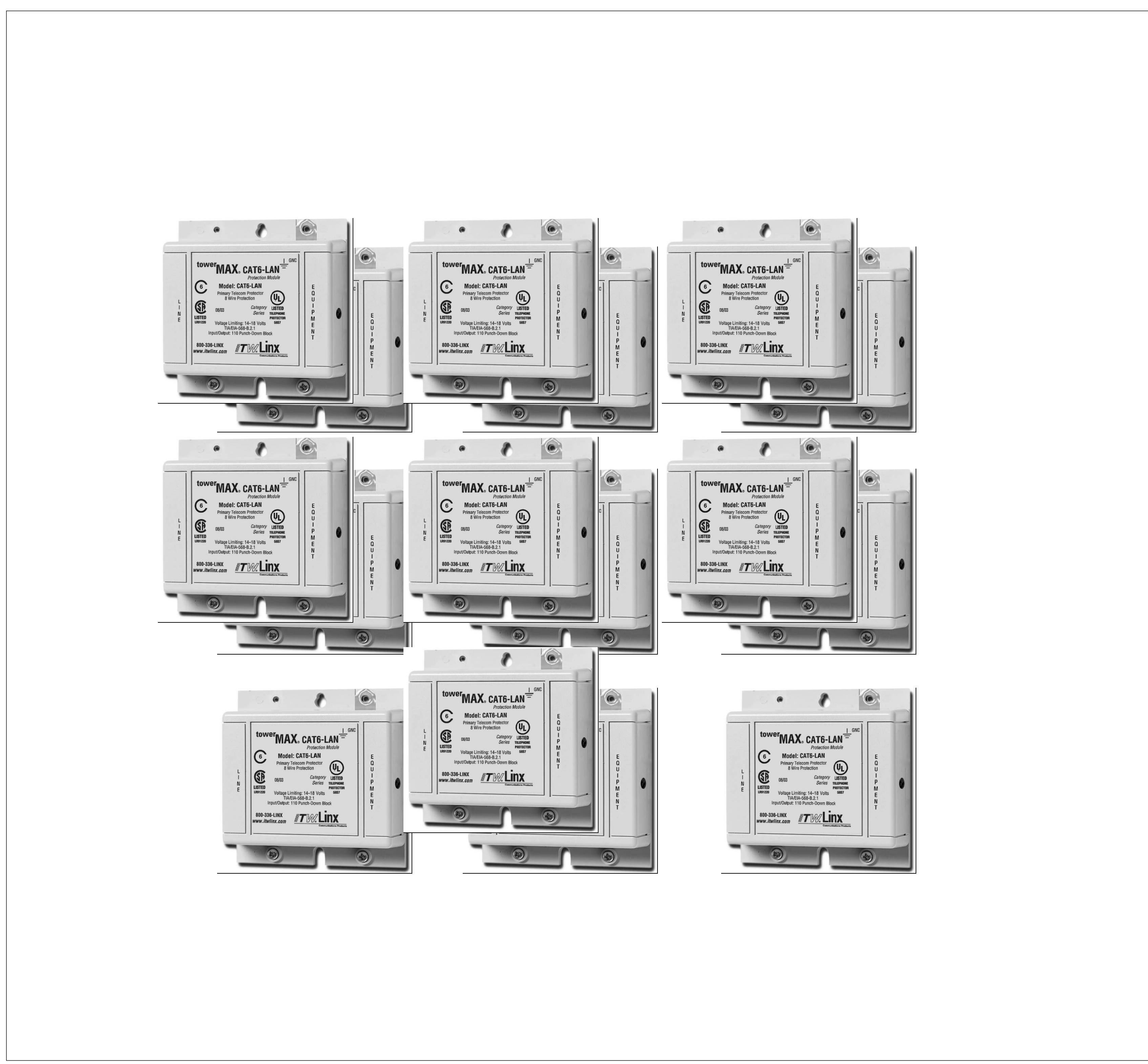
A CAT6-LAN PROTECTION MODULES SCALE: NTS
