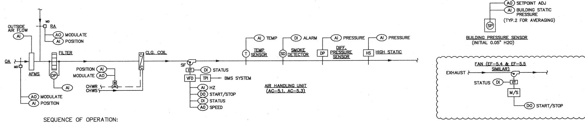
THE OPERATOR WORKSTATION / NETWORK CONTROLLER, THROUGH A USER PROGRAMMABLE SCHEDULE, SHALL ENABLE THE OPERATION OF AHU & ASSOCIATED EXHAUST FAN.
