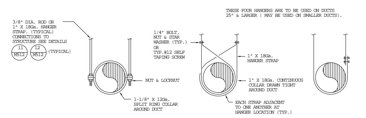
ROUND DUCT HANGER 3/8" DIA. ROD, OR 1" X 18Ga.  $\sim$  1/2" DIA. ROD. — 1" X 18Ga. HANGER HANGER STRAP, (TYP.) — (TYPICAL) STRAP, (TYP.) UNISTRUT OR 2" X 2" X 1/8 ANGLE ┌ 1" X 18Ga. OR 1 5/8" —— STRAP OVER UNISTRUT DUCT (TYP.) TOP & BOTTOM SCREWS (TYP.) ÚÞØRÁNSÖQ Ø ANÚÁHI fl ANGLE (TYP.) OR USE 1 5/8 MAX AND OVER UNISTRUT RECTANGULAR DUCT HANGER
