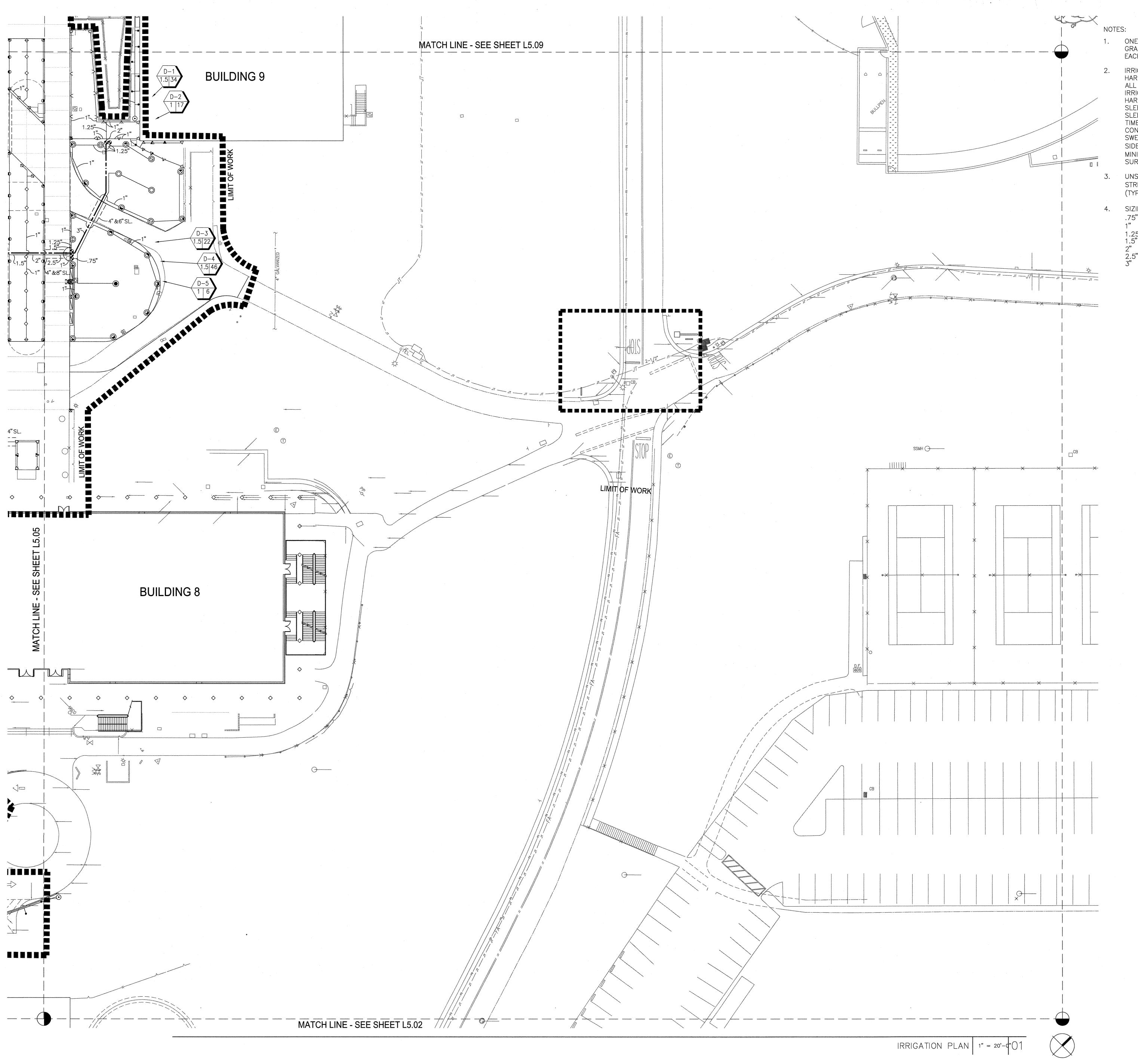
ONE BUBBLER SYMBOL IS SHOWN AT TREES FOR GRAPHIC CLARITY ONLY. INSTALL TWO BUBBLERS AT EACH TREE AS DETAILED.
