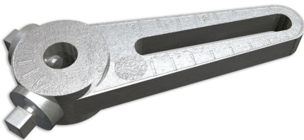
DMPR-KC051 Crank Arm, 3/8 Inch Diameter Shaft. This provides a connection from the actuator to the damper blade pin extension with a 3/8 inch diameter drive shaft, adjustable from 1 to 2-3/4 inch radius.
