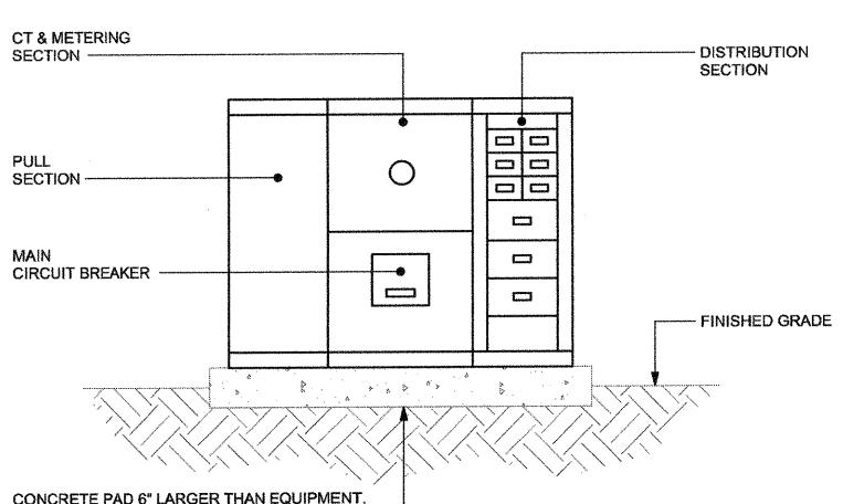
CONCRETE PAD 6" LARGER THAN EQUIPMENT, MINIMUM 3" ABOVE GRADE, 3 1/2" BELOW GRADE. PROVIDE STEEL WIRE MESH 4" GRID ———
