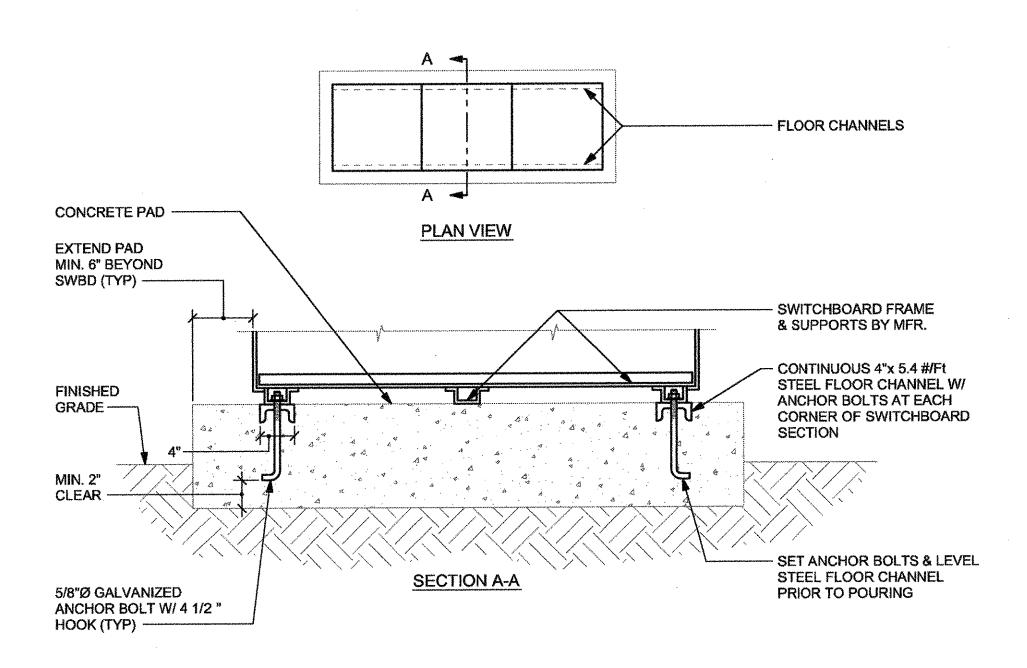
**EXTERIOR SWITCHBOARD ANCHORAGE PAD** NOT TO SCALE
