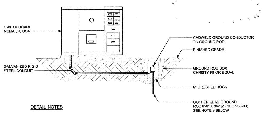
1. SIZE OF CONDUCTORS SHALL COMPLY WITH NEC TABLE 250-94.
