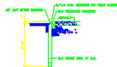
109 HEADER DETAIL SCALE 1/4"=1'-0"
