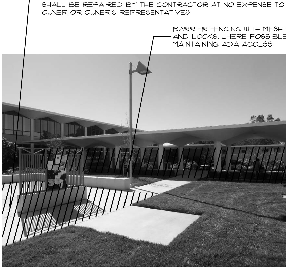
AREA FOR CONTRACTOR SETUP AND STORAGE. PROVIDE FENCING AND GATES AS REQ'D, 4' MIN. FROM EDGE OF BUILDING, WHERE POSSIBLE WHILE MAINTAINING ADA ACCESS. CONTRACTOR RESPONSIBLE FOR PROTECTION OF (E) LANDSCAPING OR (E) HARDSCAPING, INCLUDING GRASS TURF. ANY DAMAGE TO (E) LANDSCAPING OR (E) HARDSCAPING SHALL BE REPAIRED BY THE CONTRACTOR AT NO EXPENSE TO THE OWNER OR OWNER'S REPRESENTATIVES
