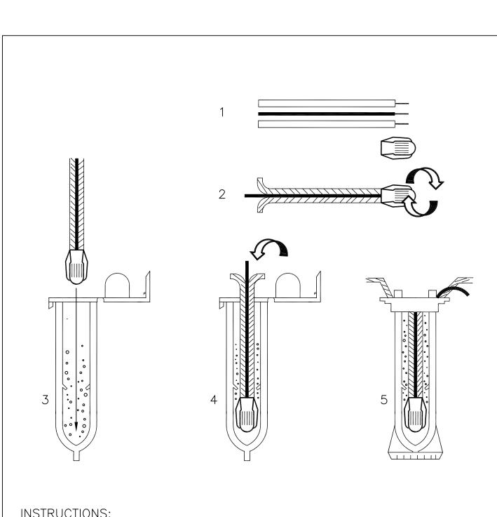
INSTRUCTIONS: 1. STRIP WIRES APPROXIMATELY 1/2" (12.7 MM) TO EXPOSE WIRE. 2. TWIST CONNECTOR AROUND WIRES CLOCKWISE UNTIL HAND TIGHT, DO NOT OVERTIGHTEN.
