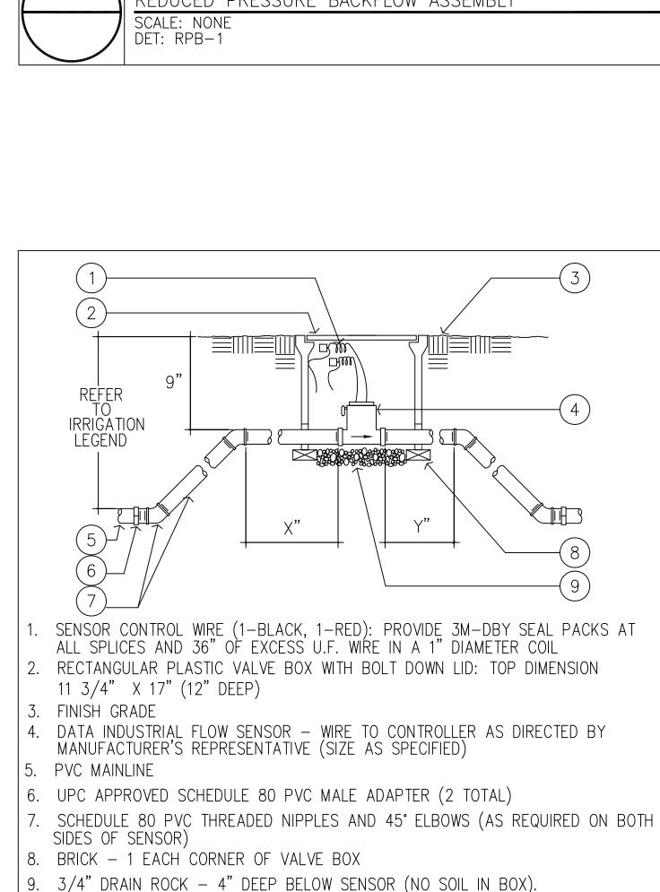
10. SENSOR WIRE FROM CONTROLLER TO VALVE BOX IS TO BE INSTALLED IN A
