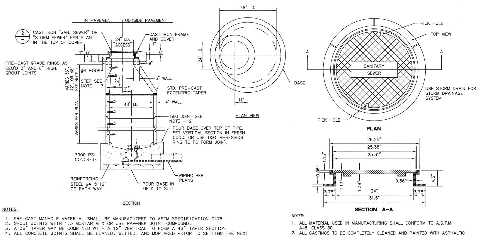
1. PRE-CAST MANHOLE MATERIAL SHALL BE MANUFACUTRED TO ASTM SPECIFICATION C478. 2. GROUT JOINTS WITH 1:3 MORTAR MIX OR USE RAM-NEK JOINT COMPOUND.
